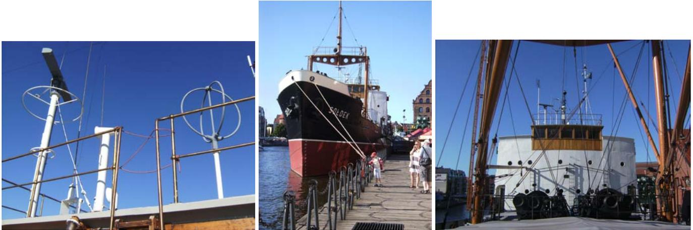
The Bellini-Tosi MF D/F loops on the monkey island are now a rare feature of a ship’s radio antenna installation – direction-finding on the marine bands not being a part of the GMDSS functional requirement.
